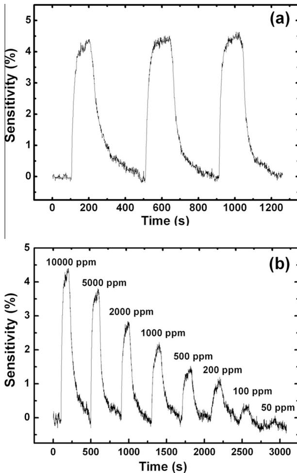
**Fig. 4 – (a) Reliable and renewable response of sensors with similar sensitivity, and proper recovery with continuous inlet of 10,000 ppm H<sub>2</sub> gas and outlet of dry air. (b) Response of sensor with continuous altering inlet gas with H<sub>2</sub> and air.**
