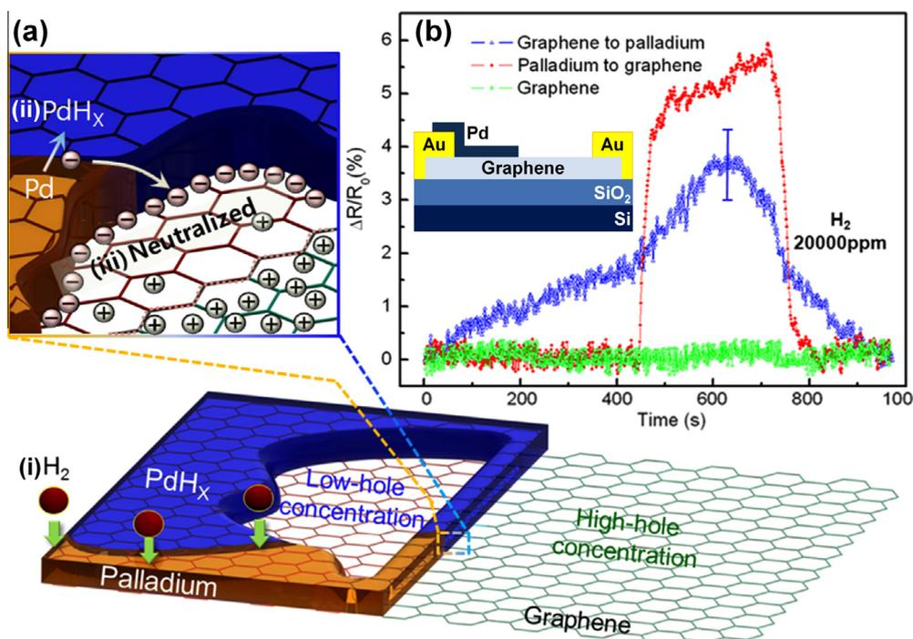
**Fig. 2 – (a) Schematics of the sensor mechanism. (b) Response of pure graphene and current-dependent graphene-Pd composite to H<sub>2</sub> gas.**
