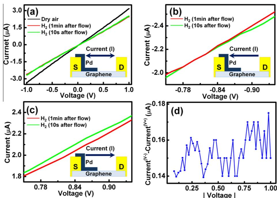
Fig. 3 – (a) I–V characteristics of the device from  $-1.0$  to  $1.0$  V. (b) I–V characteristics of the device from  $-0.92$  to  $-0.75$  V. (c) I–V characteristics of the device from  $0.75$  to  $0.92$  V. (d) Voltage–current relationship depends on current direction (y-axis represents the current flow differences between the current directions, x-axis represents the absolute voltage value).
