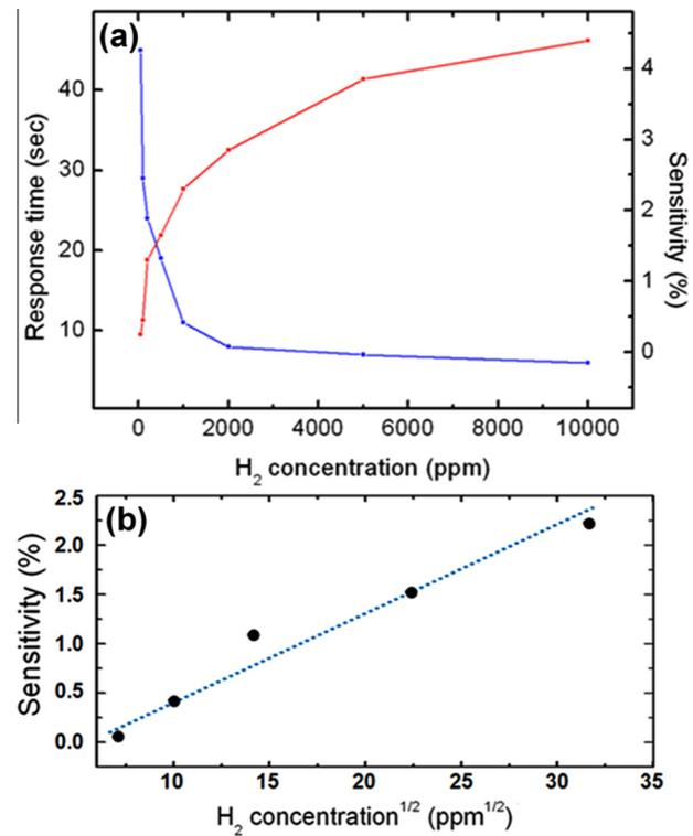
**Fig. 5 – (a) Response time and sensitivity of graphene–Pd sensor due to changing hydrogen concentration. (b) Sensor's sensitivity in low concentration (10–1000 ppm), which follows Sievert's law.**
